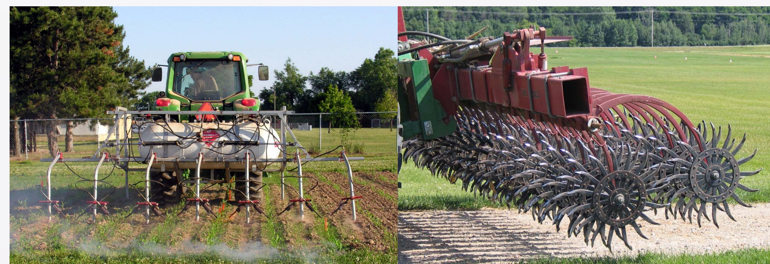
Figure 1. Propane flamer used in Objective 1 (left) and rotary hoe used in Objective 2 (right).
